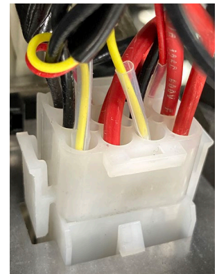
Figure 12: Split vat fryer with attached tilt switch wiring. Polarity is not a factor.
