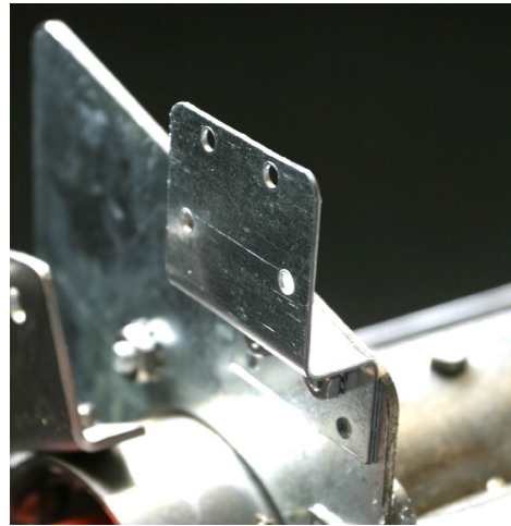
Figure 3: The switch bracket is shown installed on the outer side of the element assembly. Mount it with the short side down, using the provided short screws. See Figures 4-7 for specific position mounting.
